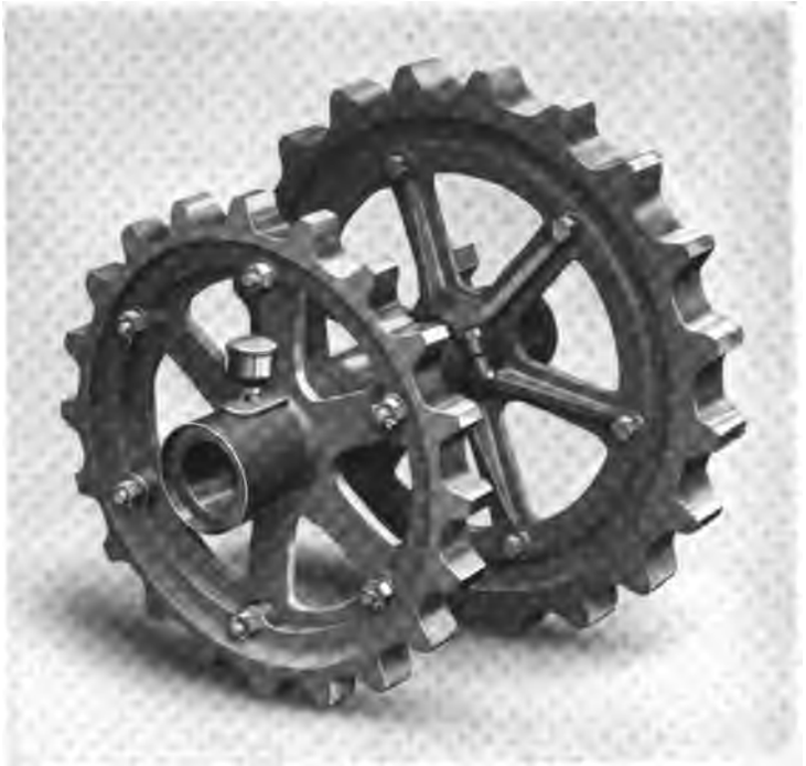
Fig. 46. Flange Journal with sprockets bolted in place
