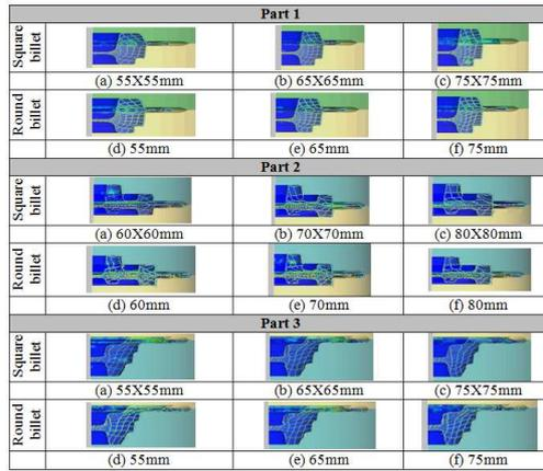
Figure 1: Comparison of Metal Flow With Different Billet Sizes and Shapes
